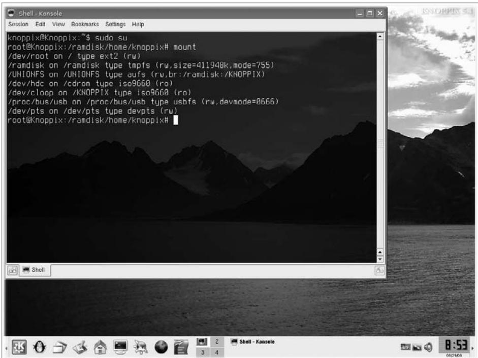
**Figure 14-12.** Knoppix doesn't load your server's file systems automatically.
